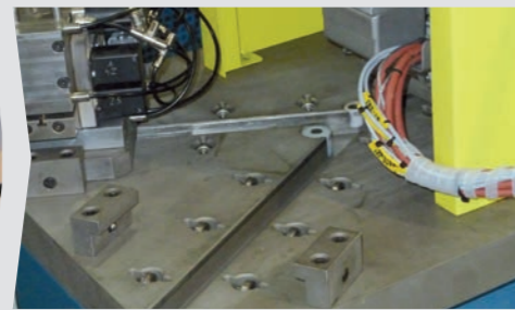
Y-table with partially open safety gate, two-hand operation and BG approval
